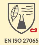
Protective clothing certified by EN ISO 27065, should be labelled with a pictogram of a conical flask with a leaf.
